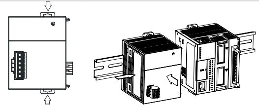
EN Clip up the two DIN rail clip on the module. Parallel the module groove on the back to the DIN rail, then push and slide along until hearing a click.
