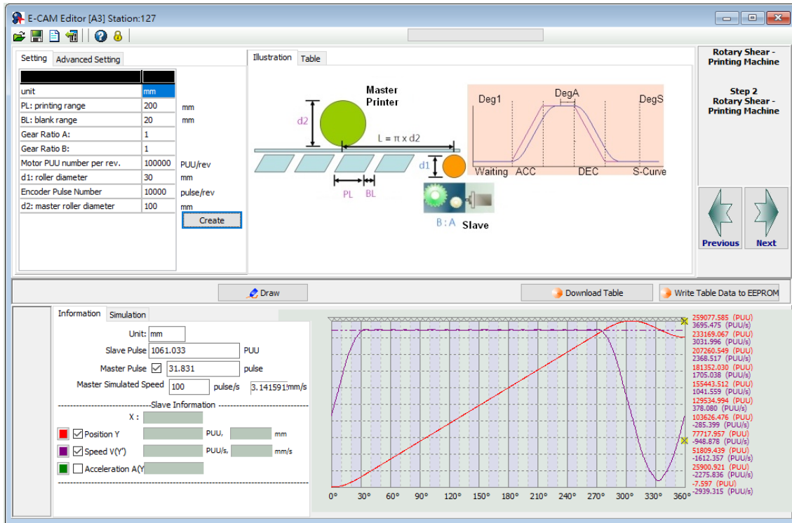
Figure 7.3.7.14 ASDA-Soft rotary shear - intermittent printing machine setting interface
