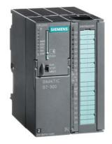
SIMATIC S7-300, CPU 312C Compact CPU with MPI, 10 DI/6 DQ, 2 high-speed counters (10 kHz) Integr. power supply 24 V DC, work memory 64 KB, Front connector (1x 40-pole) and Micro Memory Card required
