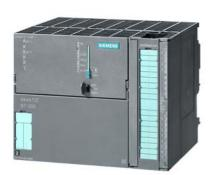
\*\*\*Spare part\*\*\* SIMATIC S7-300, CPU 317T-2 DP, Central processing unit for PLC and Technology tasks, 1024 KB work memory, 1st interface MPI/DP 12 Mbit/s, 2nd interface DP (drive), Integr. I/O for technology Front connector (1x 40-pole) and Micro Memory Card min. 8 MB required
